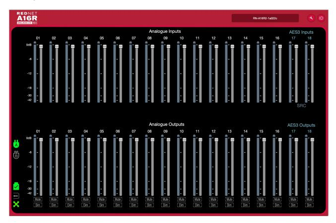
The image shows the Level control sliders, level meters and the Mute/Dim buttons for each of the 18 inputs and outputs.
