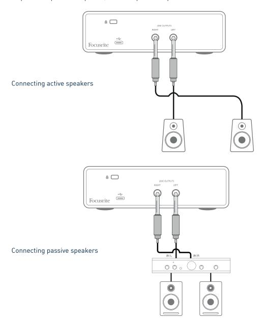
The line outputs are 3-pole (TRS) ¼" (6.35 mm) jack sockets, and are electronically balanced. Typical consumer (Hi-Fi) amplifiers and small powered monitors will have unbalanced inputs, either on phono (RCA) sockets, or via a 3.5 mm 3-pole jack plug intended for direct connection to a computer. In either case, use a suitable connecting cable with jack plugs at one end.
