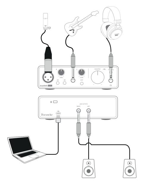
This setup shows a typical configuration for recording using DAW software on your Mac or PC. You would record vocals through Input 1 and guitar through Input 2 into your recording application, while monitoring the playback via headphones.
