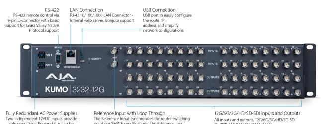
safe operations. Power status can be checked from a LAN attached browser point per SMPTE specifications. The Reference Input supports Blackburst for SD and tri-level sync for HD
