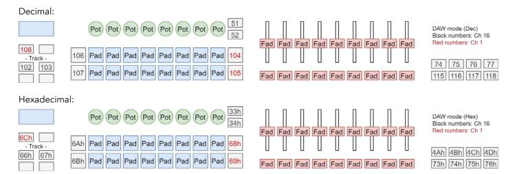
To provide some degree of script compatibility with the Launchkey Mini [MK3], the Scene Up and Scene Down buttons also report back CC 68h (104) and 69h (105) respectively on Channel 16.
