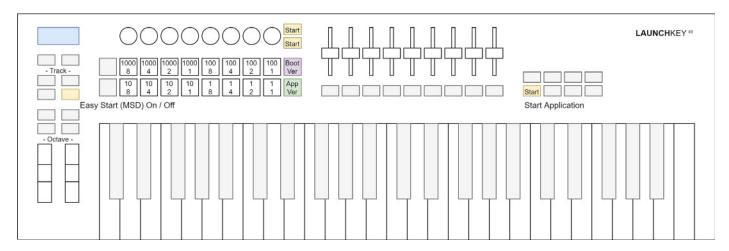
The Fixed Chord button toggles Easy Start mode between On and Off. When Easy Start is ON, the Launchkey [MK3] shows up as a Mass Storage Device to provide a more convenient first-time experience. You can turn this off once you are familiar with the device to disable this Mass Storage Device.
