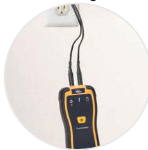
Traces on de-energised circuits
